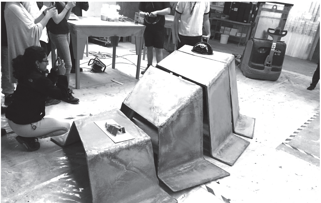
Figure 3: Pop-up Surfaces. Top: concrete still in 'pop-up' molds, Bottom: Final folded forms (Photo by author).
